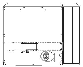
**Step 3.** Attach co-axial air-inlet duct to rear of fireplace (6 screws).
